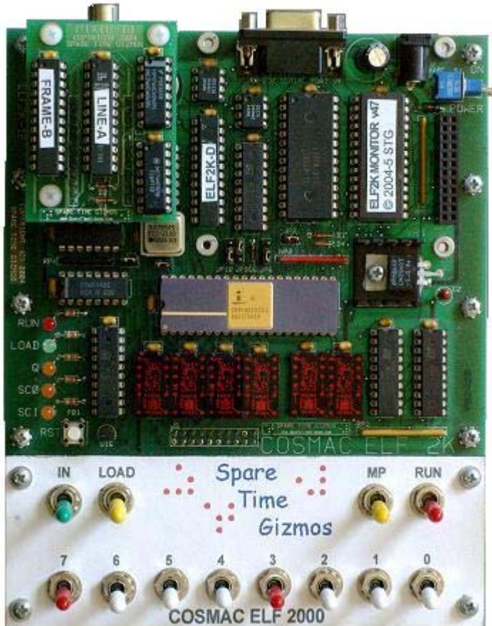
Photo 11 - STG1861 installed on the ELF 2000
